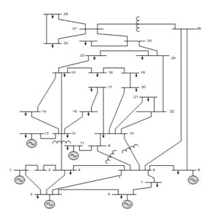
Fig .2 Single line diagram of IEEE-30bus [2]
